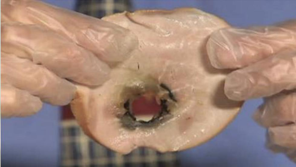
***The burning effect of a button battery when placed between slices of ordinary ham, simulating a child's throat.***
